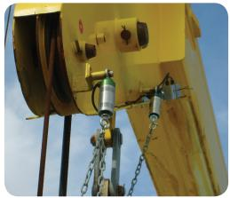
The most versatile mechanical A2B Switch, featuring a user replaceable switch mechanism and a built in 4.7K resistor for seamless integration.
